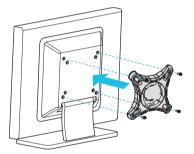
3. Mount the DeskMini 110 series by turning it counterclockwise.
