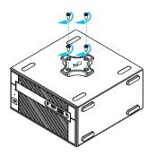
2. Attach the other VESA Bracket to the rear of a compatible display using the four screws.
