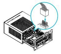
2. Align the motherboard tray with the two sliding tracks on the chassis while sliding it back to the chassis.
