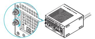
3. Connect the two WiFi 2.4/5 GHz Antennas to the antenna connectors. Turn the antenna clockwise until it is securely connected.
