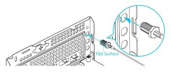
2. Fasten the screw nuts to secure the antenna connectors.
